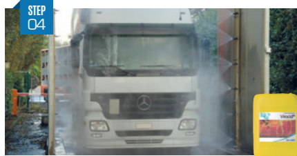
STEP 04 Disinfect (spray or foam) Disinfect all surfaces inside and out with the right disinfectant. Work your way down from the top to the bottom and pay attention to cracks and wheels. Do not forget the underside of the vehicle. Dilution: 0.25 - 0.5%.
