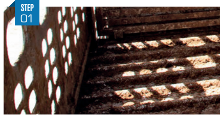
STEP 01 Dry clean after unloading Take away the remaining dirt.
